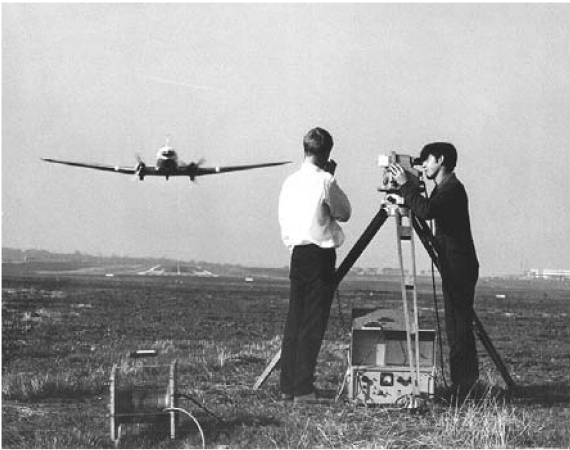
Fig. 1 The two surveyors on the ground measure the aircraft's deviation from the desired flight path using a theodolite (ILS Calibration by DC3, http://www.airwaysmuseum.com/DC3%20ILS%20calibration.htm [retrieved 13 December 2006]).
